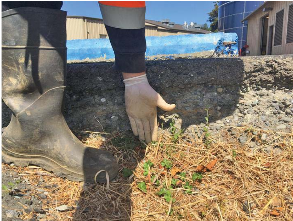
Photo 3: Vertical drop at landslide scarp
